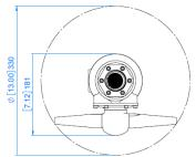
INLET PRESSURE INLET 11/2" BSPP
