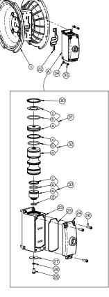
f. Unscrew the Allen screw (28) using suitable key. Open cover (26) & replace O-ring (27) with new one.
